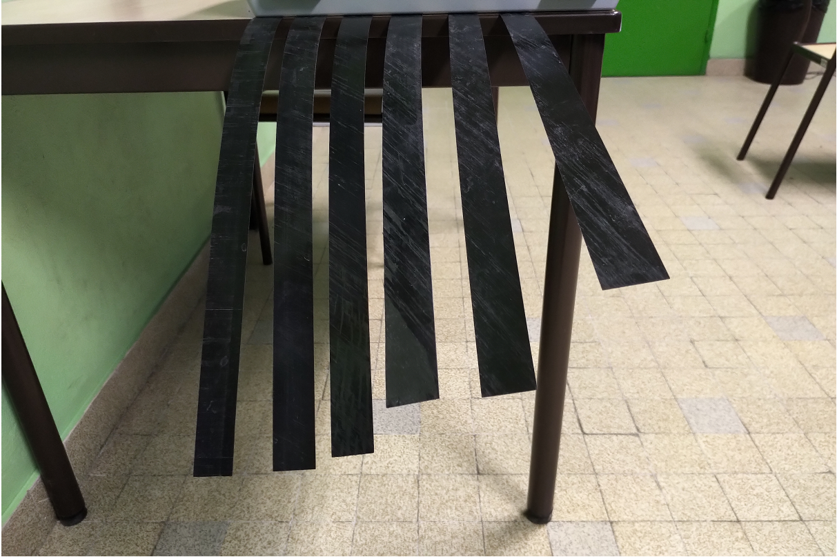
Figure 12: Laminate static deflection, from left to right : [90, 0, 90] , [60, 0, 60] , [45, 0, 45] , [30, -30, 30] , [30, 0, 30] and [15, 0, 15] .
