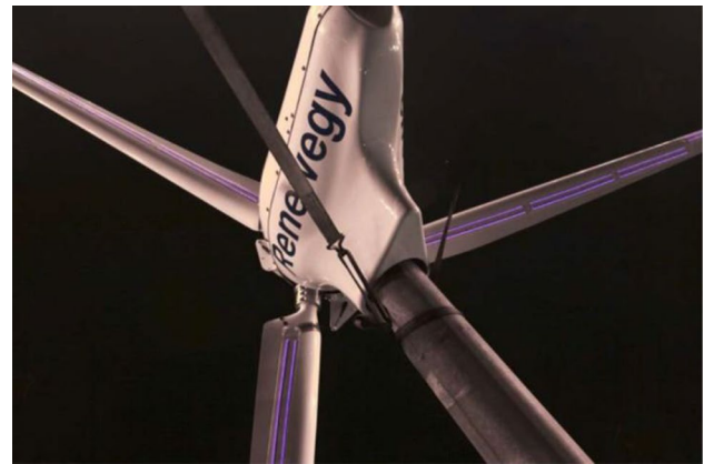
Fig. 5 Renewegy VP-20 wind turbine with retrofit plasma actuators on the blade’s suction side Original figure 26 reproduced from Cooney et al. (2016); reprinted by permission of the American Institute of Aeronautics and Astronautics, Inc
