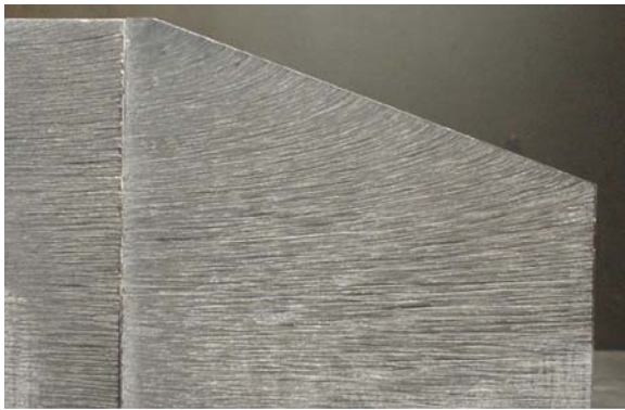
Fig. 19c Friction line visualisations on the side of the rear window. \theta = 20^\circ , V_0 = 30 \text{ m.s}^{-1}
