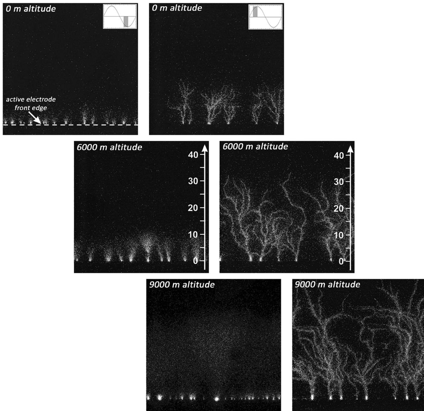
Fig. 1. Development of surface filaments during the (left plots) cathode and (right plots) anode half period of a DBD operating at different altitude conditions (scale in millimeters).
