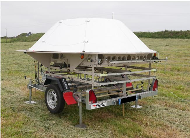
Figure 3: The SODAR (SONic and Detection And Ranging) device used for the onshore kite measurements.
