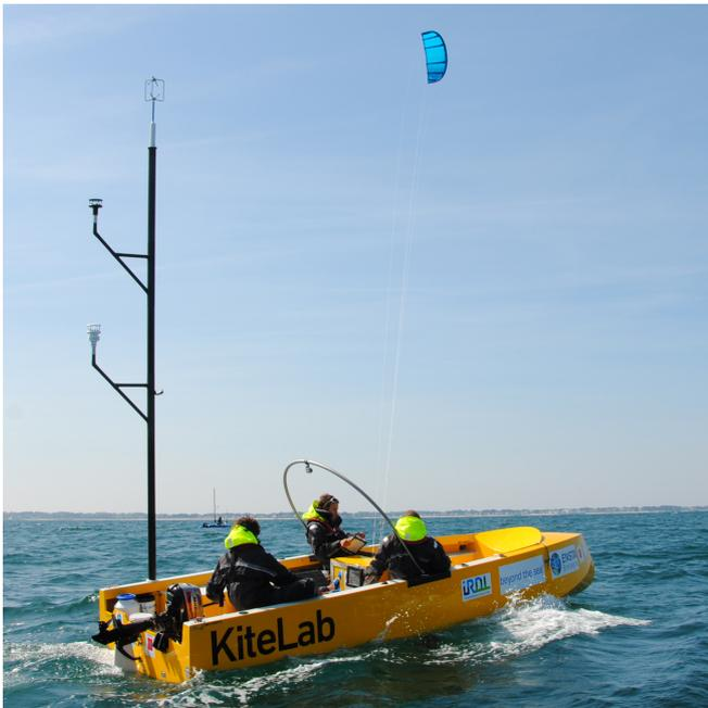
Figure 1: Picture of the KiteLab, the experimental platform specifically designed to carry out measurements on effects and performances of kite propulsion. The 5-meter wind measurement mast is visible on the rear of the boat. The inflatable kite flying over the boat is a 5m<sup>2</sup> one.
