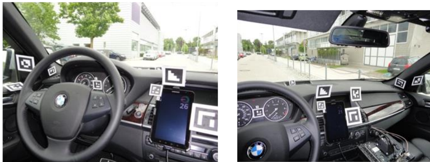
Figure 1. Attachment of the nomadic device and the markers in the test vehicle
