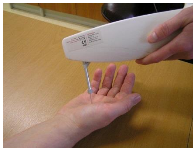
Figure 6, 7. Myometer for muscles stiffness measurements
