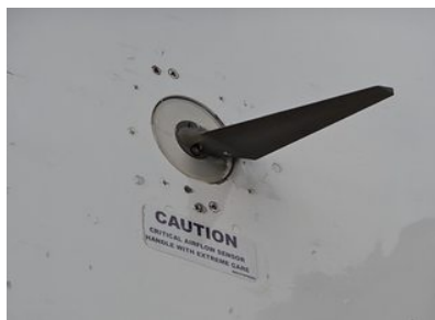
FIGURE 7. \alpha -vane employed usually to measure the angle-of-attack.
