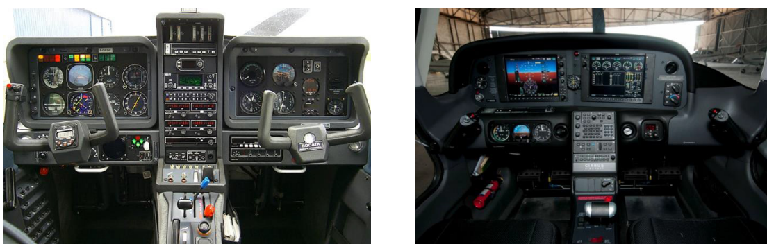
Figure 1. Cockpit analogique (gauche) vs glass cockpit (droite)
